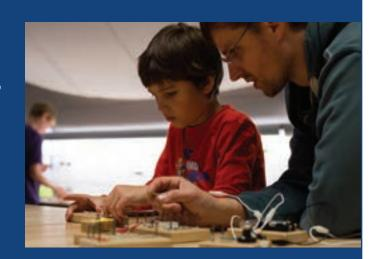
Remember, your switch must include a *conductor*—a material that lets electricity flow through the circuit.
